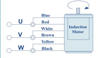
For the Voltage 230 VAC, 3-Phase Supply, Wires are connected as shown in the fig.
