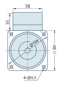
90 Watt: AC Geared Motor With Lead wires
