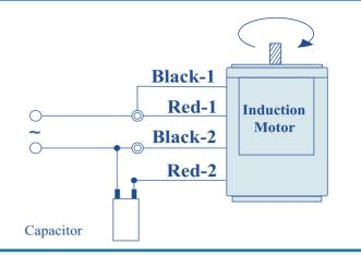
Black Wires are for Starting purpose and Red wires for the Running purpose, as shown in fig.,
